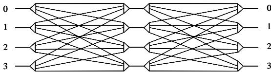
Fig. 4. The structure of strictly nonblocking VSB (4,4) network.
