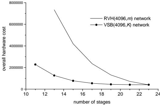
Fig. 10 Overall hardware cost of RVH(4096,  $m$ ) network and VSB(4096,  $K$ ) network of various stages.
