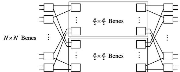
Fig. 5 Recursive definition of an  $N \times N$  Benes network.
