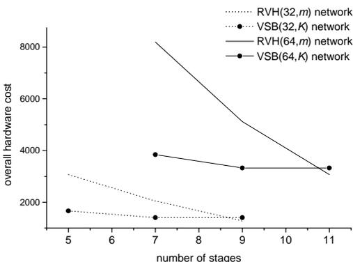
Fig. 11 Overall hardware cost of networks of sizes  $N=16$  and  $N=32$ .
