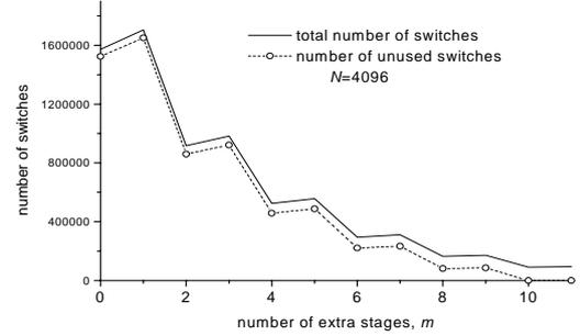
Fig. 2. Total number and the number of unused SEs in a  $4096 \times 4096$  RVH( $n,m$ ) network with different extra stages.
