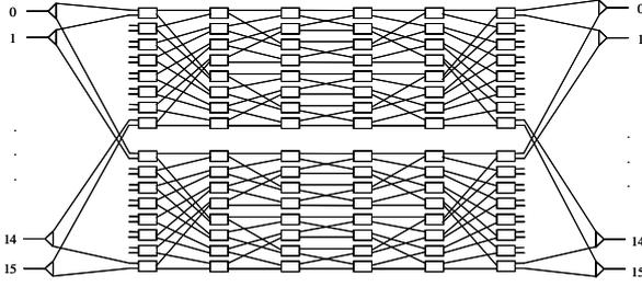
Fig.1 The construction of a VH (4,2,2) network from banyan networks.
