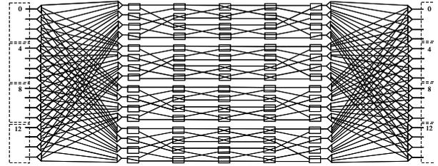
Fig. 9 Crosstalk-free realization of permutation (10) in a VSB(16,4) network.
