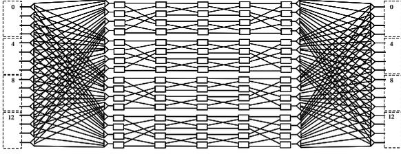
Fig.3 The construction of a VSB (16,4) network from  $8 \times 8$  Benes networks.
