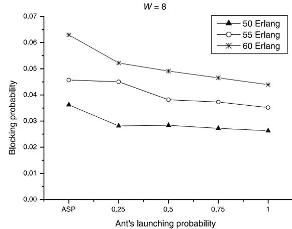
Fig. 5 Performance gain of HABR with difference value of ant's launching probability in compare with ASP on the NSF network.
