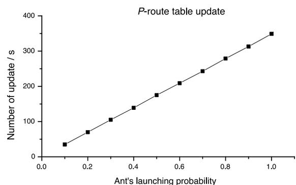
Fig. 8 Number of updates for a  $P$ -route table versus ant's launching probability when  $t = 1$  ms, EON network.
