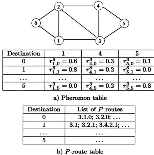
Fig. 1 A simple network and its routing tables of node 3.
