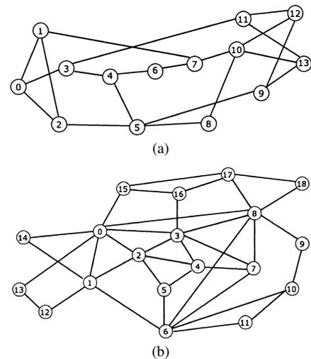
Fig. 3 Network topologies: (a) NSF network with 14 nodes and 21 links. (b) EON network with 19 nodes and 35 links.
