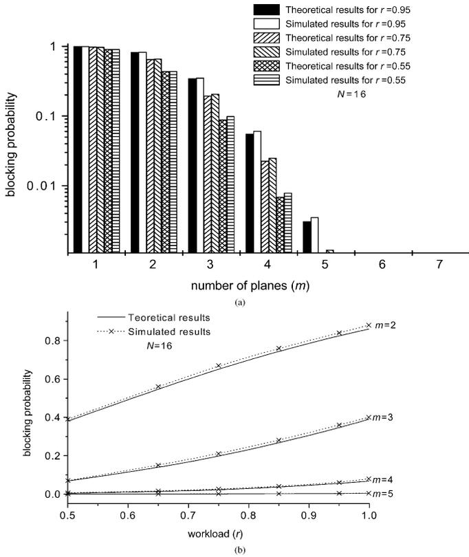
Fig. 5. Blocking probability of VSPB(16, *m*) network. (a) Blocking probability versus *m* with  $r = \{0.55, 0.75, 0.95\}$ . (b) Blocking probability versus *r* with  $m = \{2, 3, 4, 5\}$ .
