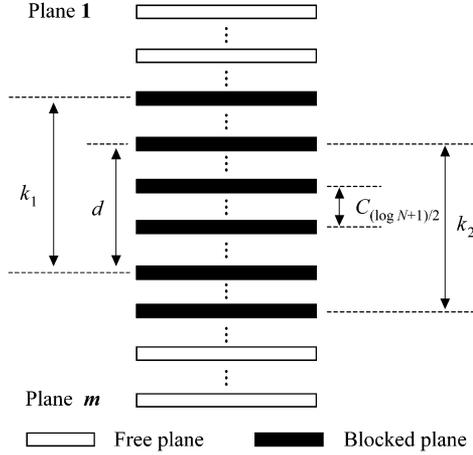
Fig. 2. VSPB( $N, m$ ) with  $k_1$  planes blocked in the first half of the tagged SEs,  $k_2$  planes blocked in the second half of tagged SEs, among them a total of  $d$  blocked planes are overlapped.
