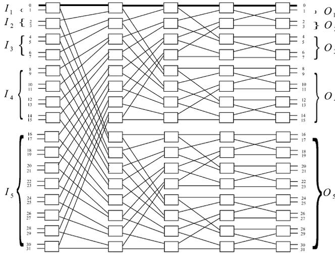
Fig. 1. A  $32 \times 32$  Banyan network (odd number of stages).
