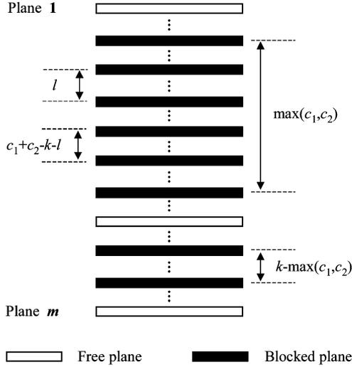
Fig. 4. VSPB  $(N, m)$  with  $c_1$  connections passing through the first tagged SE,  $c_2$  connections passing through the second tagged SE, among them  $l$  connections passing through both tagged SEs, and there are a total of  $k$  planes ( $\max(c_1, c_2) \leq k \leq kc_1 + c_2 - l$ ) blocked.
