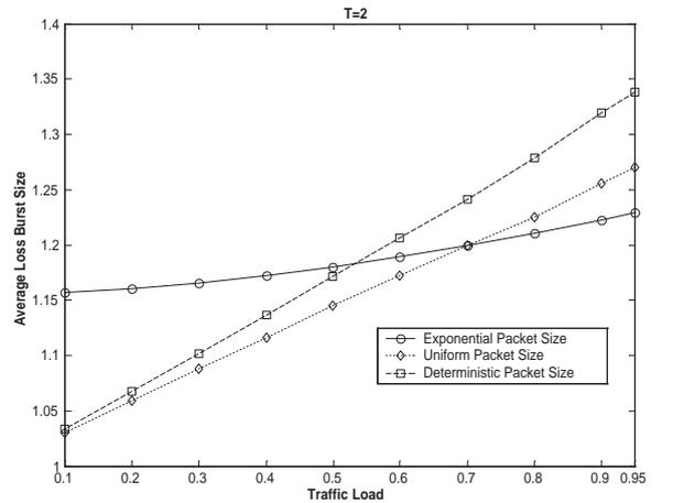
(b) Average loss burst size vs. Traffic load when  $T=2$
