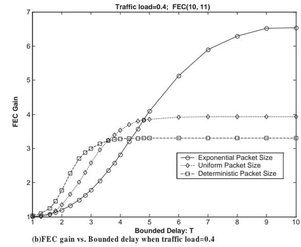
(b) FEC gain vs. Bounded delay when traffic load=0.4
