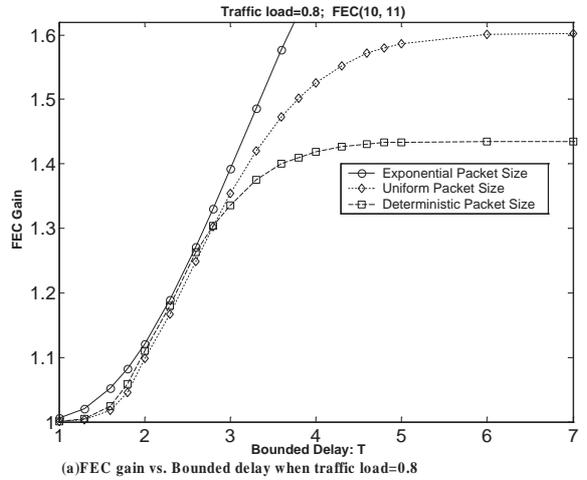
(a) FEC gain vs. Bounded delay when traffic load=0.8
