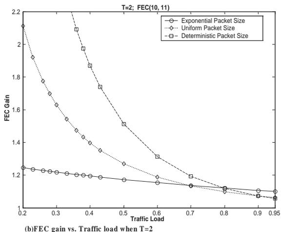
Fig. 5. FEC gain Vs. Traffic load under different bounded delay
