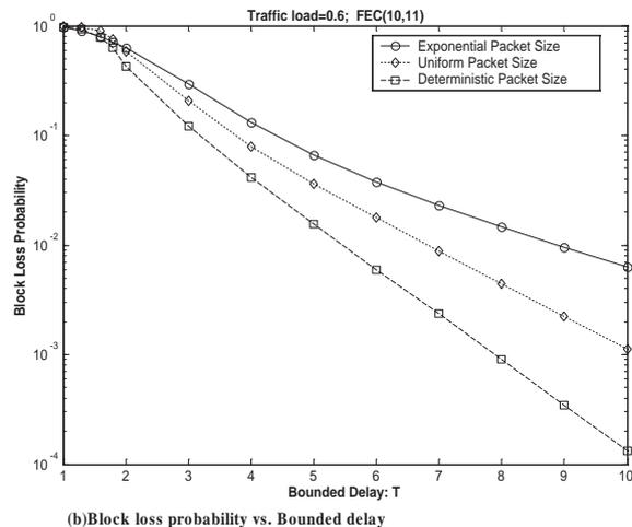
(b) Block loss probability vs. Bounded delay
