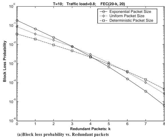
(a) Block loss probability vs. Redundant packets
