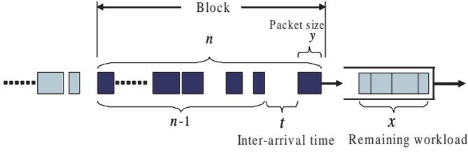
Fig. 1. Queueing model of the packet loss process
