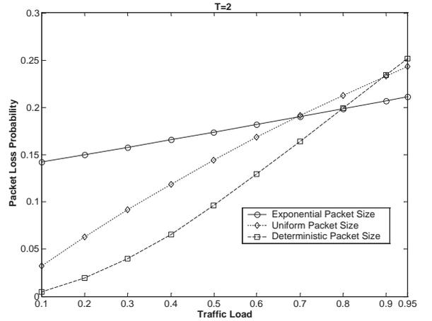
(a) Packet loss probability vs. Traffic load when  $T=2$
