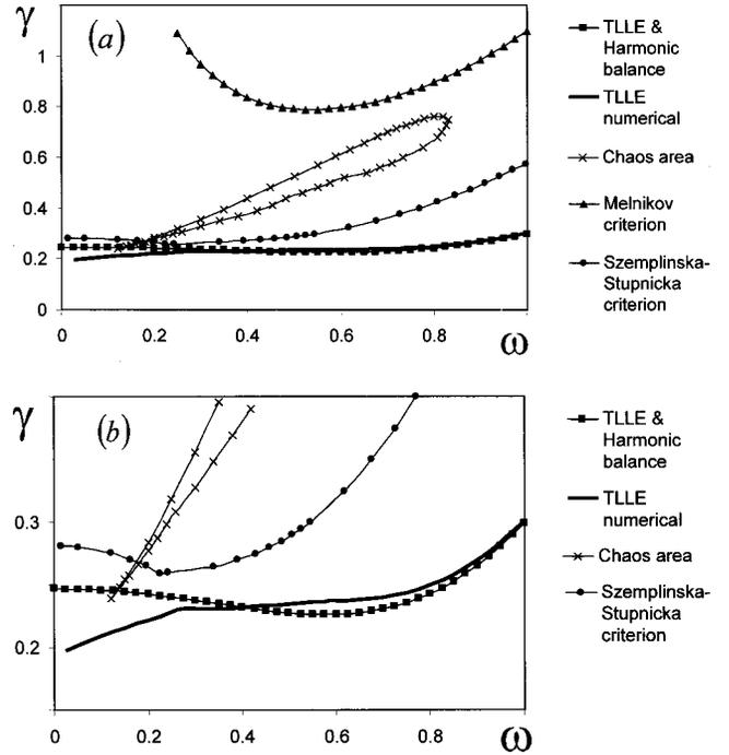
FIG. 6. State diagram of the double-well Duffing oscillator (54) at  $\alpha = \beta = \frac{1}{2}$ ;  $\delta = 1$  (a) and its blow-up (b).
