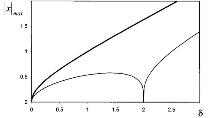
FIG. 2. Size of the asymptotic stability area vs dissipation parameter  $\delta$  for the hard-mode Duffing oscillator at  $\omega_0 = 1$ ,  $\varepsilon = 1$ . The application of TLLE together with optimized linear coordinate transform results in a larger area of asymptotic stability (heavy line) compared to the case of the system with diagonalized matrix of the linear part (light line).
