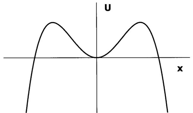
FIG. 3. Potential function for Duffing equation with soft-type nonlinearity.
