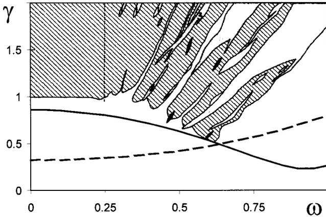
FIG. 7. Comparative performance of the proposed method, i.e., the combination of harmonic balance and TLLE analysis (solid line), and Melnikov criterion (dashed line) for the pendulum oscillator (71). The areas of chaotic behavior are hatched (from Ref. [51]).
