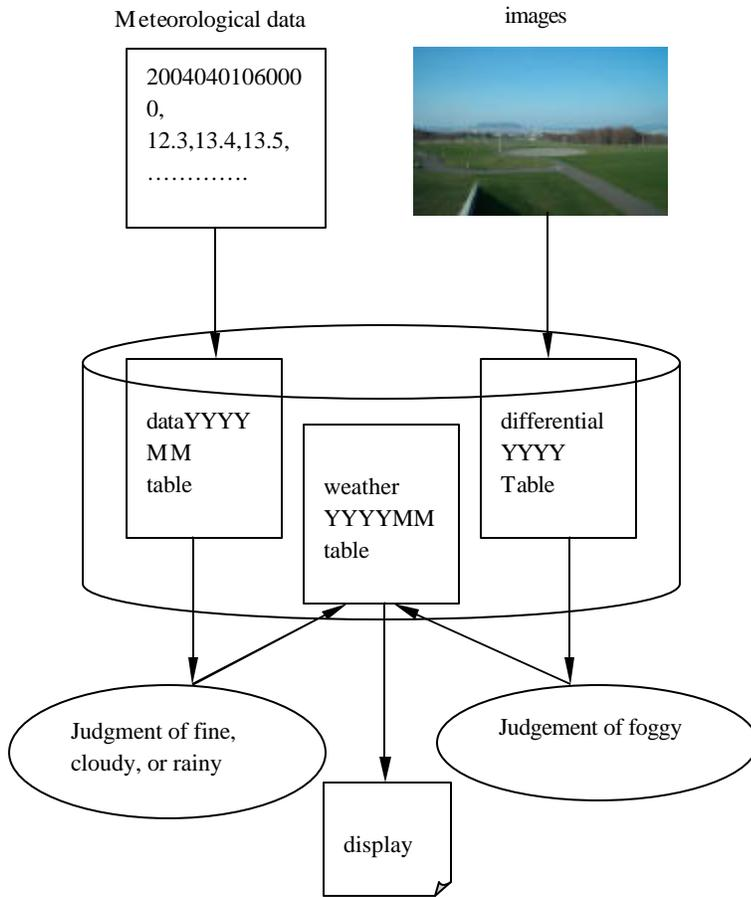
**Figure 2 Design concept for weather retrieval system.**
