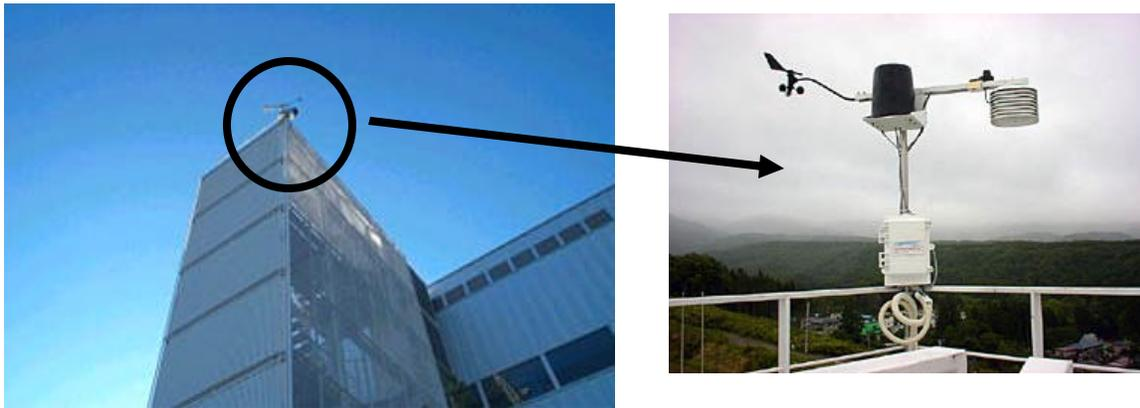
(a) Sensor module for meteorological observation.
